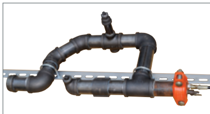
Burst pressure testing of DI threaded fittings (2')
